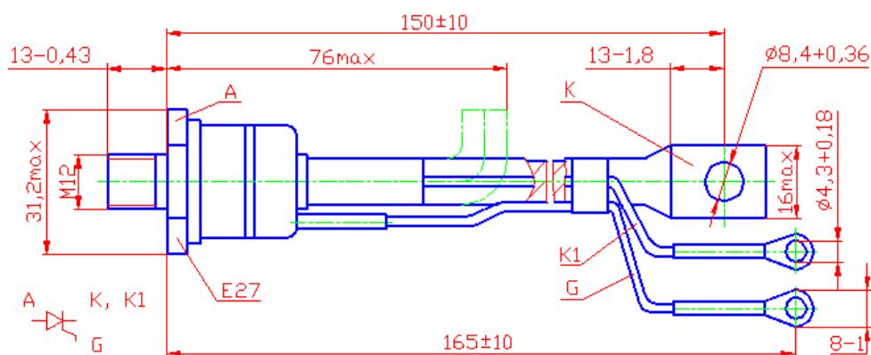
Tightening torque : 12 ÷ 18 Nm
